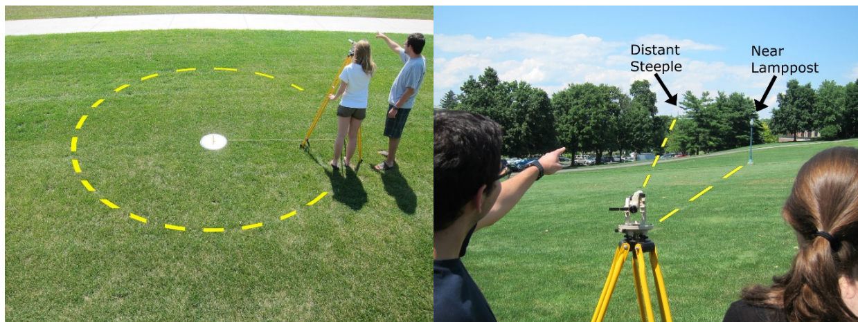
Figure 2. Students trace out a two-meter radius circle to mimic the Earth’s orbit around the Sun (left). Then they measure the direction to nearby objects from several locations along the circle. Using a surveyor’s transit, students measure the direction to a nearby lamp post, using the direction to a distant landmark as a reference (right).
