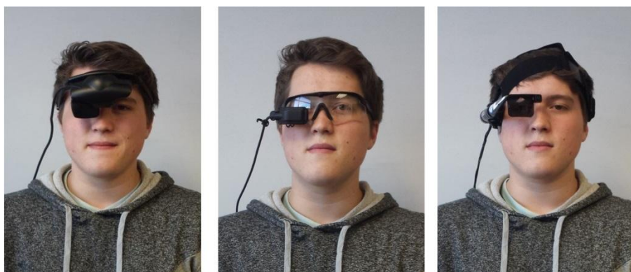
Figure 3. The three HMDs used in evaluations. The displays are all monocular and include fully occlusive on the left, partially occlusive in the middle, and see-through with a half-silvered mirror on the right. Monocular displays were used to maximize the amount of light reaching the eye.
